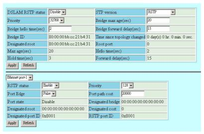
Figure 6-8 Rapid Spanning Tree Protocol Setting Dialog
